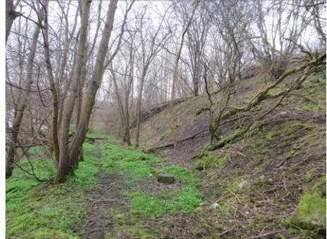
The level area is only presently wide enough for the existing Right of Way (around 1 - 1.5m). Any widening to Cycling by Design Standards would require both earthworks and slope retention. The long fall along the path is also relatively steep, and further earthworks would be required to meet the required standards. These earthworks would evidently have an impact on existing woodland vegetation.
